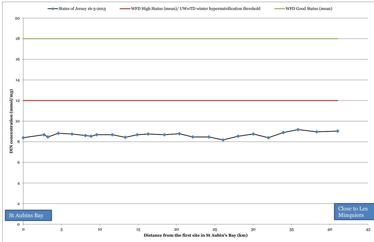
**Figure 3.2** shows that dissolved inorganic nitrogen (DIN) levels along the transect are relatively constant, remaining between 8-9 mmol/m<sup>3</sup>. Transitional and Coastal (TRAC) waterbody WFD DIN thresholds are shown for information. These levels are adequate for healthy growth of *Ulva* but remain just below the level associated elsewhere with prolific growth.
